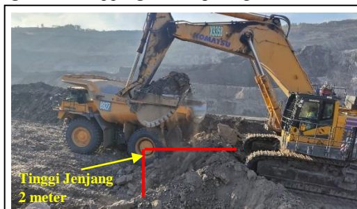
Gambar 3. Tinggi jenjang excavator loading material ripping
