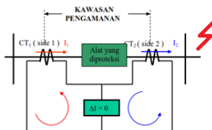
Gambar 3. Kondisi Gangguan Luar Differential Relay [1]
