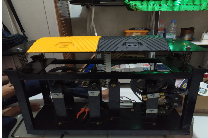
Gambar 1. Road Power Generator
