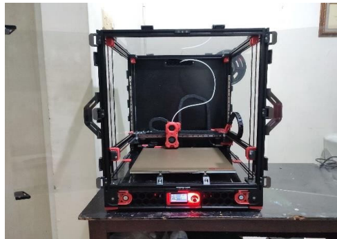
Gambar 1. Mesin 3D Printing tipe Voron 2.4 350mm
