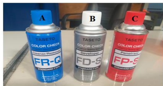
Gambar 14: Cleaner / Remover (A), Developer (B), Liquid Penetrant (C)
