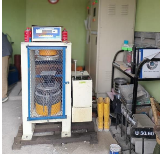
Gambar 2. Alat Tes Tekan Compression Testing Machine di PT. Intidi Beton Jatim.
