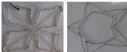
Gambar 3. Rangka Lampu Hias Dililit Led Strip
