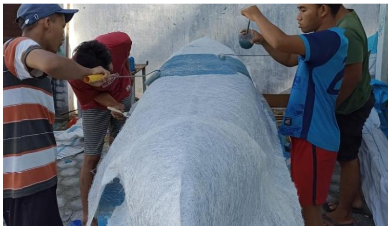
Gambar 7. Pelapisan Fiberglass Reinforced Plastic (FRP)
