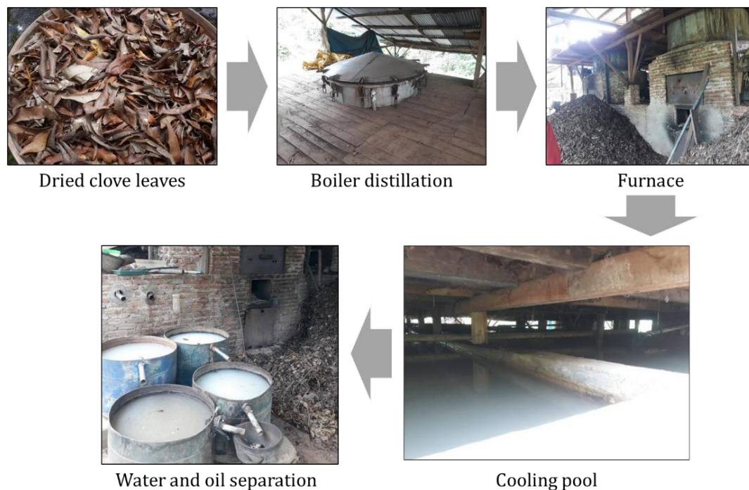
Figure 2. Dried clove leaf extraction process
