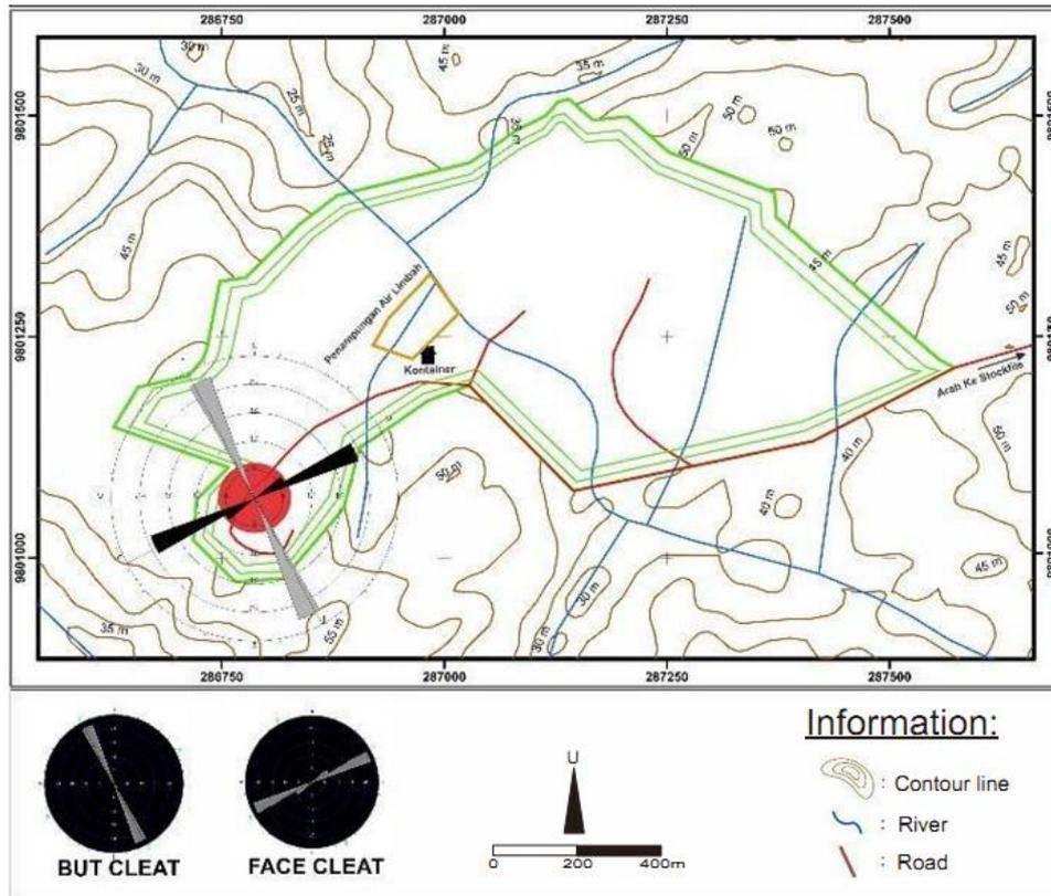
Figure 8. Map of Stress Direction Based on Analysis of Cleat Measurement Data
