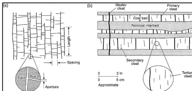
Figure 1. Geometric features of coal cleats. (a) cleat pattern on a horizontal plane (b) cleat pattern based on cross-section [6].
