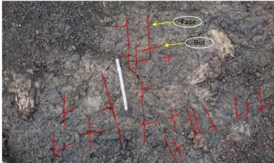
Figure 6. Face Cleat and But Cleat in research area
