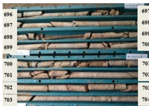
Figure 5. The core sample of 480 – 488 meter depth as an example of the breccia layers
