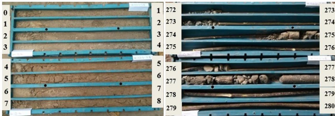
Figure 1. The core sample of 0 – 8 meter depth as an example of the soil layers (left), The core sample of 272 – 280 meter depth as an example of the conglomerate layers (right)
