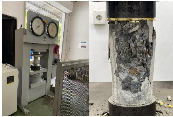
Figure 5. Compressive Strength Test of Concrete
