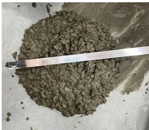
Figure 4. Slump Flow Test of Concrete
