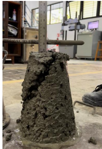
Figure 3. Slump Test of Concrete
