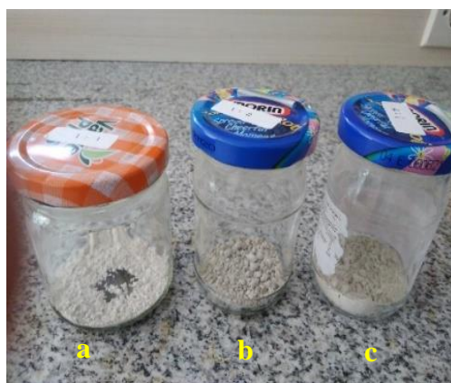
Figure 3. CaO/K 2 O calcined with ratio: 1:1 (a), 1:2 (b), dan 2:1 (c)
