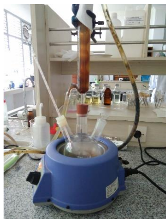
Figure 4. Transesterification of Castor Oil by Reflux Method
