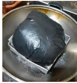
Figure 11. heating a plastic bag on an aluminum plate on a gas stove fire [6], [7]
