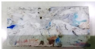
Figure 12. a) white abstract printed surface b) equilateral rectangular board measuring 35mm x 35mm x 11mm
